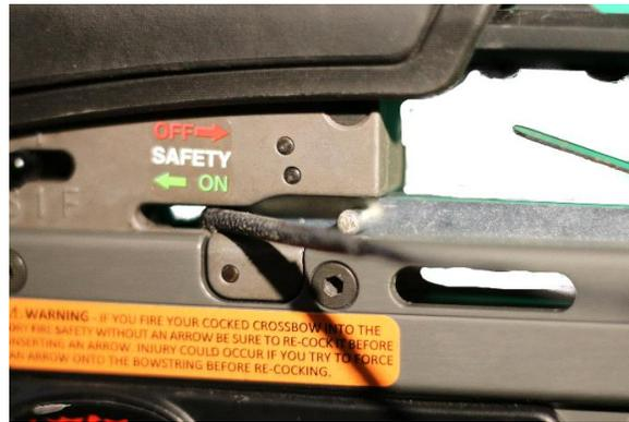
5) Pointing in a safe direction, take the safety off and squeeze the trigger. You will hear a click. Your serving is now being supported by the Crossbow Defuser. Holding the crossbow by the foregrip with one hand, and pointing in a safe direction, unscrew the T knob with your dominant hand until the string and serving are in the defused/neutral position. Unscrew the T knob just slightly more, slide back 1/2", tighten, and lift off.
